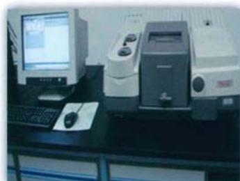
Fourier transform infrared spectrophotometer
